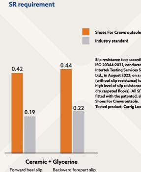
Slip resistance test according to EN ISO 20344:2021, conducted by Ltd., in August 2022; on a scale of 0.0 high level of slip resistance, e. g. on dry carpeted floors). All SFC shoes are fitted with the patented, slip-resistant Tested product: Carrig Low 62201.
